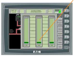
LCD display showing load amperage detail
